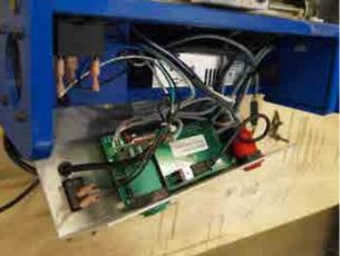
Route the z-zero plate and alligator clip wires through the electronics enclosure bulkhead port.
