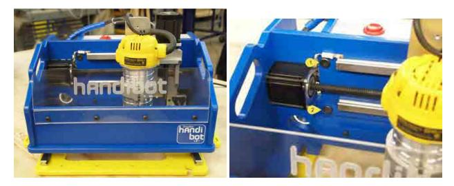
With power off, manually push the X-axis to the right of the tool. For easier access, it may be helpful to remove the clear debris shield on the front of the tool. Two bolts for the electronics enclosure bulkhead are located near the X-axis motor. Use the 4mm hex key to remove these bolts.
