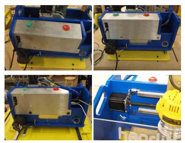
Carefully rotate the electronics enclosure cover back into position being sure to tuck all wires into position. Insert the left side of the plate into the slot on the Handibot body. Check again for any protruding wires, and then slide the right side of the cover past the enclosure bulkhead. Push the bulkhead slot over the cover. Replace the 5 bolts with a 4mm hex wrench.
