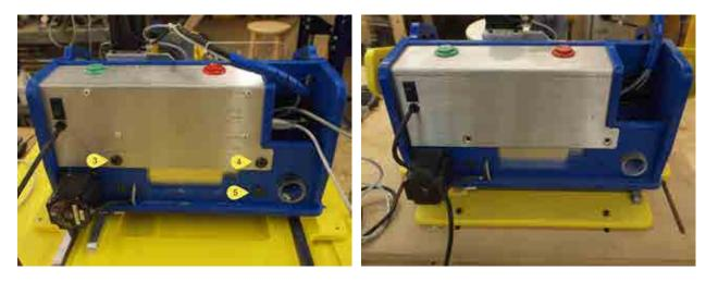
Three bolts on the reverse side of the tool that must be removed. Remove the two bolts from the electronics enclosure cover. The remaining electronics enclosure bulkhead bolt is next to the vacuum port.
