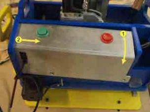
Push the electronics enclosure bulkhead to the side until the cover is released from the slot. Pull the right side of the enclosure out and to the right.
