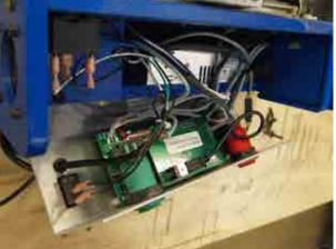
Once the enclosure cover is released from the slots rotated the top away from the Handibot. Be careful not to excessively strain any wires. This exposes the control card, control board, powers supply and other components critical to Handibot operation.
