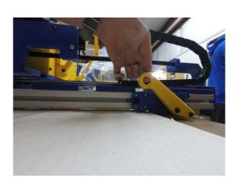
Slide the tool until the "current position" pointer is lined up with the mark that you made before releasing the clamps on the frame. This will ensure that you've made an exact 6" move along the material.
