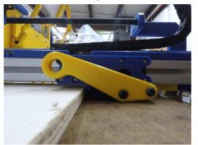
After your first cut in a series of tiled cuts—make a mark on the material through the groove of the "next position" marker.
