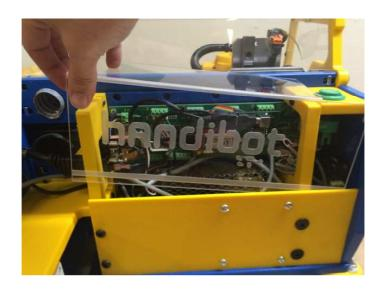
Secure cover in place using red handled hex key.
