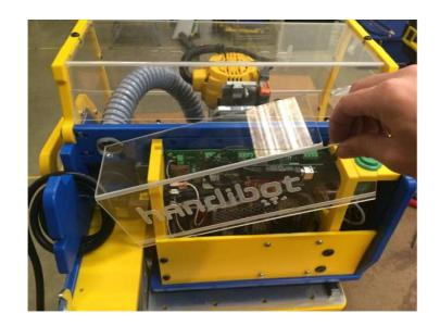
7 To get access to the spindle control terminals we'll need to temporarily remove the control card. Start by unplugging the ribbon cable.
