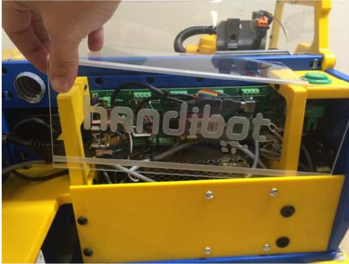
**13** Secure cover in place using red handled hex key.
