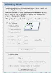
Check the "Tile Toolpaths" box to open the options below...you'll most often be using "individual tiles". The tile width and height should be set equal to the cutting area of your tool. For the Handibot Adventure Edition, this is 6" x 8" and for the Large Sheet Tool, this is 6" x 24". Leave "Tile Overlap" at 0.0
