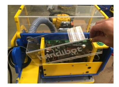
Older control cards will be held in place by two screws. Remove the two phillips head screws holding the FabMo control card in place. Gently pull the FabMo card off of the interface board.
