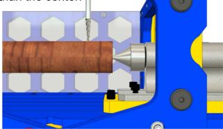
To accomplish a "tiled" cut, release the red toggle clamps and shift the T-slot tray by 4 inches in either direction. Lock the clamps into the v-shaped grooves to precisely locate the work piece for your next cut.
