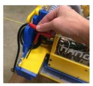
Clip wire tie and disconnect the OTG cable from the A-D converter and remove the converter.
